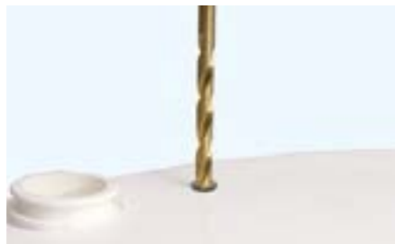
Carefully drill a 10mm hole in the lid of the unit where indicated in the instructions
