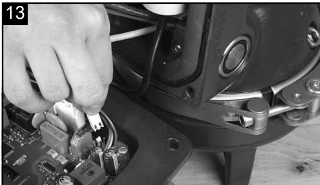
Fix the capacitor wire on the PC board.
